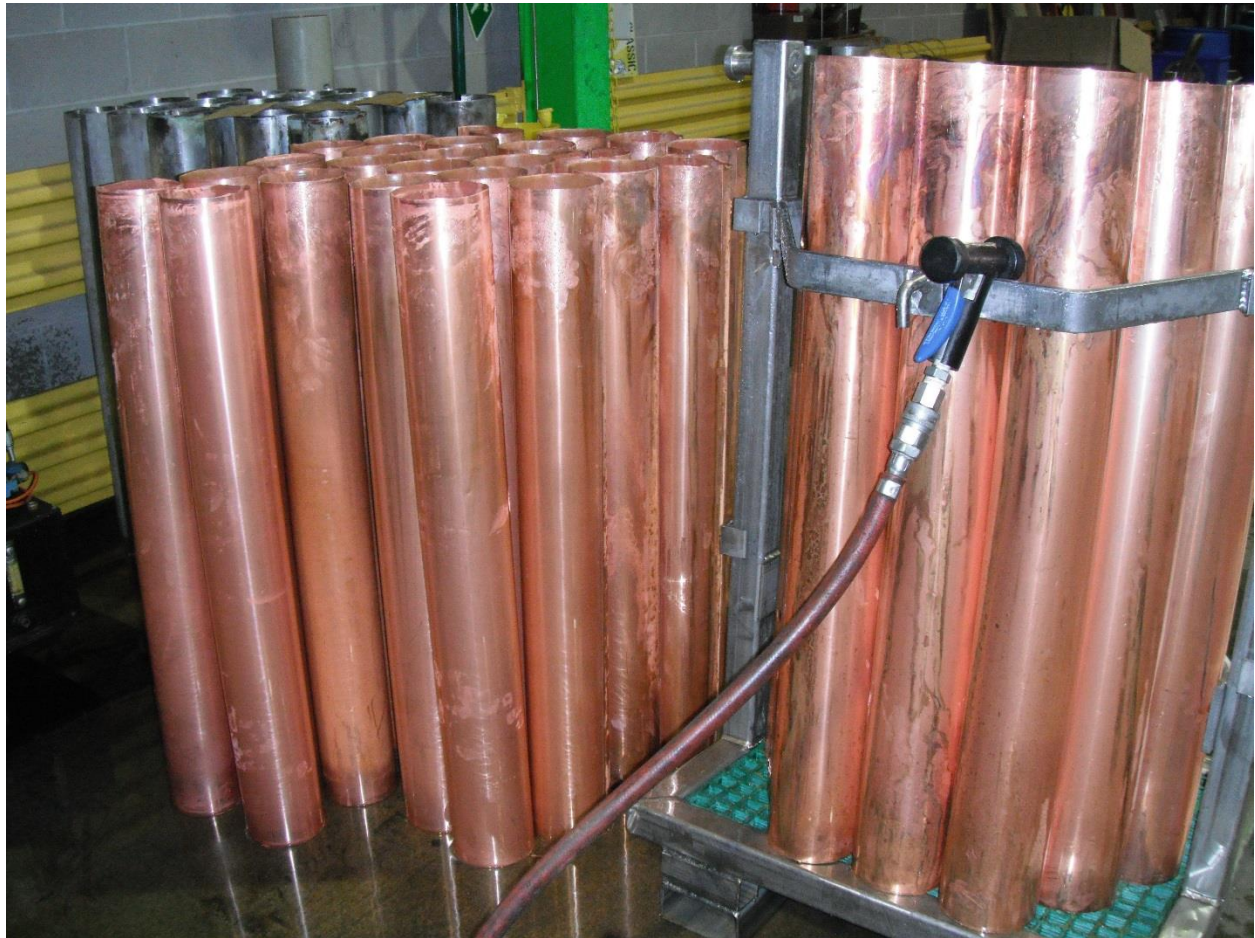
Illustration 2: Copper Cathode recently pulled from the pilot testing in White Pine.
