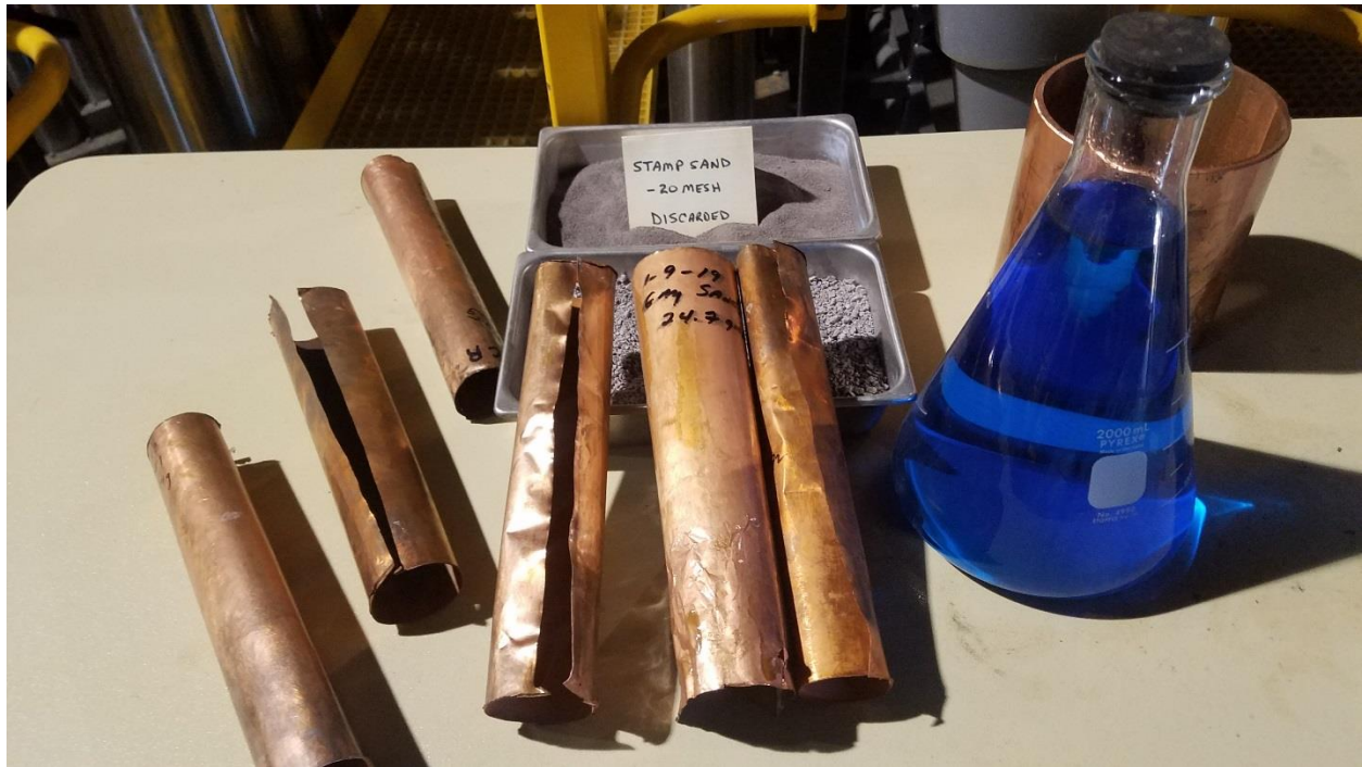
Illustration 1: Copper Cathode recovered from Stamp Sands at White Pine Copper Refinery.
